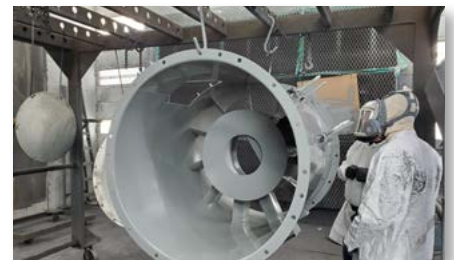
Powder Coating Paint System
