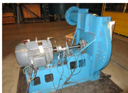
Mechanical Run Testing
