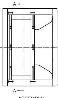
The new Aero Acoustic Diffuser™ is exclusively available on the Twin City Fan E-Series plug type plenum fans. The patented design allows the plug type plenum fan to discharge sound power reductions by up to 3dBA while increasing aerodynamic static efficiency by up to 4%.
