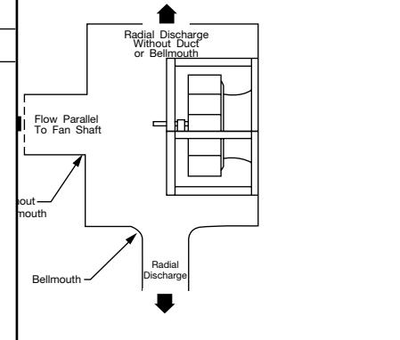
**Example:** A system requires 14.15 m<sup>3</sup>/sec at 1250 Pa static pressure at standard air density with one 1250 mm diameter duct with bell-mouth placed in a radial discharge. Determine RPM and absorbed power:
