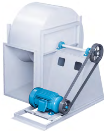
Arrangement 9F Belt Drive Extended Structural Frame to Mount Motor Not suitable for spring isolators
