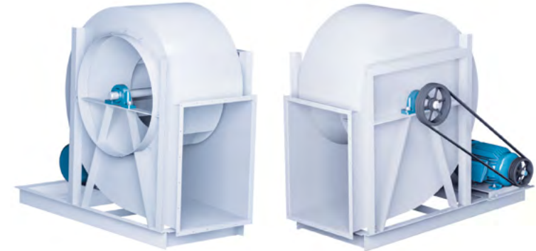
Arrangement 3F Belt Drive Extended Angle Frame to Mount Motor (Fan welded to frame/base - typically not suitable for spring isolators)
